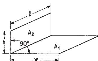
Two finite rectangles of same length, having one common edge, and at an angle of  $90^\circ$  to each other.
