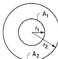
Concentric cylinders of infinite length.
