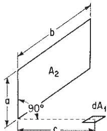
Plane element  $dA_1$  to rectangle in plane  $90^\circ$  to plane of element.
