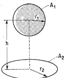
Sphere of radius  $r_1$  to disk of radius  $r_2$ ; normal to center of disk passes through center of sphere.
