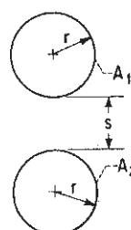
Infinitely long parallel cylinders of the same diameter.
