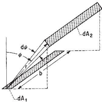
Strip of finite length  $b$  and of differential width, to differential strip of same length on parallel generating line.
