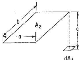
Plane element  $dA_1$  to plane parallel rectangle; normal to element passes through corner of rectangle.
