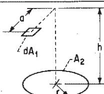
Plane element  $dA_1$  to circular disk in plane parallel to element.
