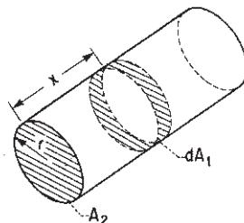
Ring element  $dA_1$  on interior of right circular cylinder to circular disk  $A_2$  at end of cylinder.
