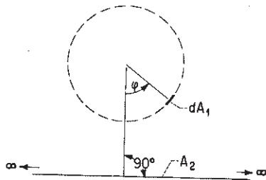
Element of any length on cylinder to plane of infinite length and width.
