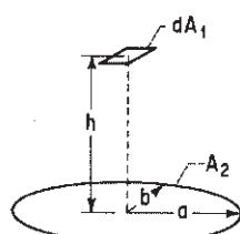
Plane element  $dA_1$  to elliptical plate in plane parallel to element; normal to element passes through center of plate.
