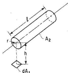
Plane element  $dA_1$  to right circular cylinder of finite length  $l$  and radius  $r$ ; normal to element passes through one end of cylinder and is perpendicular to cylinder axis.
