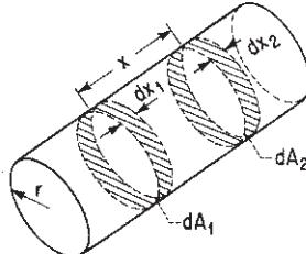
Two ring elements on the interior of a right circular cylinder.
