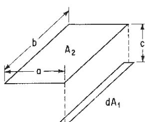
Strip element to rectangle in plane parallel to strip; strip is opposite one edge of rectangle.
