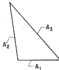
Infinitely long enclosure formed by three plane areas.
