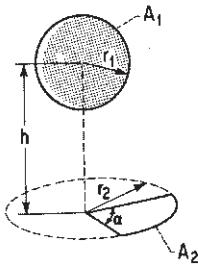
Sphere to sector of disk; normal to center of disk passes through center of sphere.
