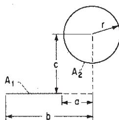
Infinitely long plane of finite width to parallel infinitely long cylinder.
