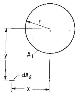
Strip element  $dA_2$  of any length to infinitely long cylinder.
