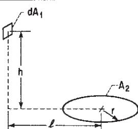
Plane element  $dA_1$  to circular disk; planes containing element and disk intersect at  $90^\circ$ .
