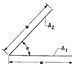
Two infinitely long plates of equal finite width  $w$ , having one common edge, and at an included angle  $\alpha$  to each other
