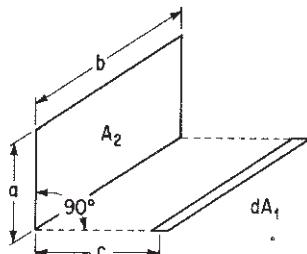
Strip element  $dA_1$  to rectangle in plane  $90^\circ$  to plane of strip.
