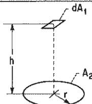
Plane element  $dA_1$  to circular disk in plane parallel to element; normal to element passes through center of disk.
